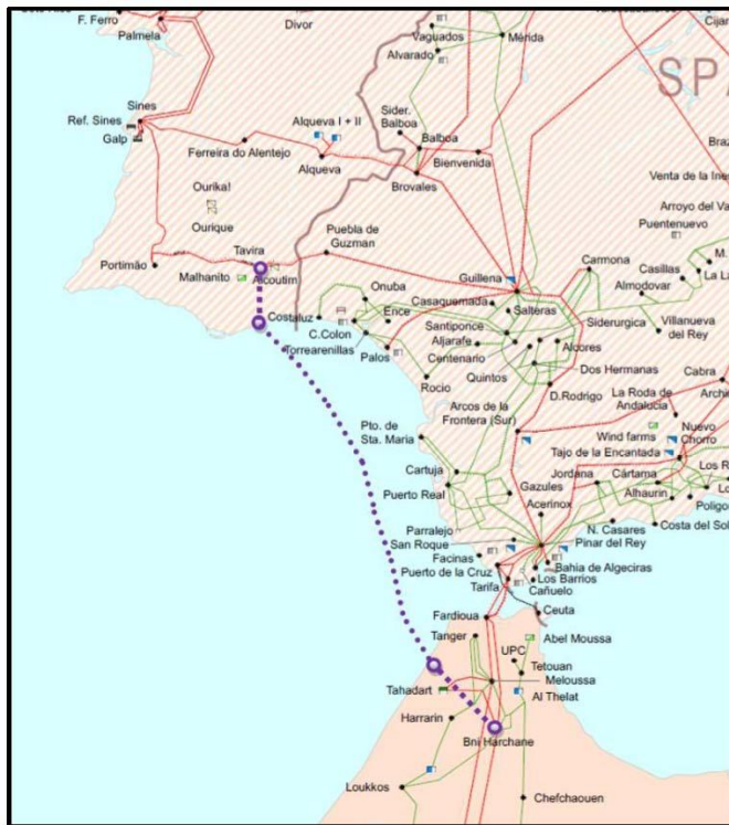
Figure 2. Morocco-Europe – MAPT existing interconnections and projected (in dash-line) source: https://www.med-tso.com/ .
