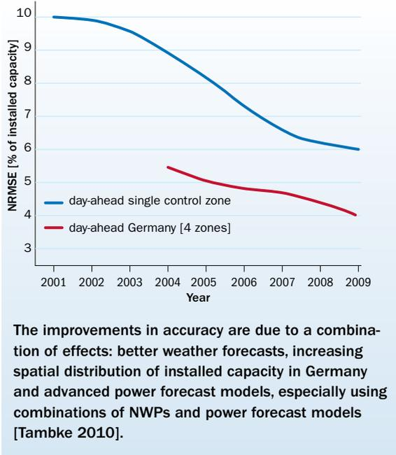
FIGURE 14: IMPROVEMENT OF FORECAST ACCURACY BY USING ENSEMBLE PREDICTIONS
